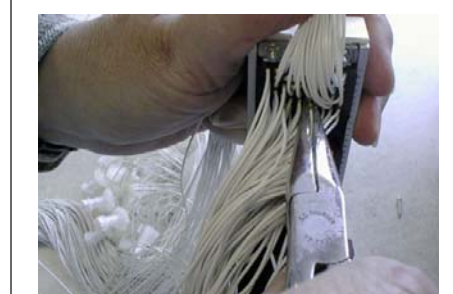
Figure 9-11. Use a pair of needle-nose pliers to grip the contact and pull it out
