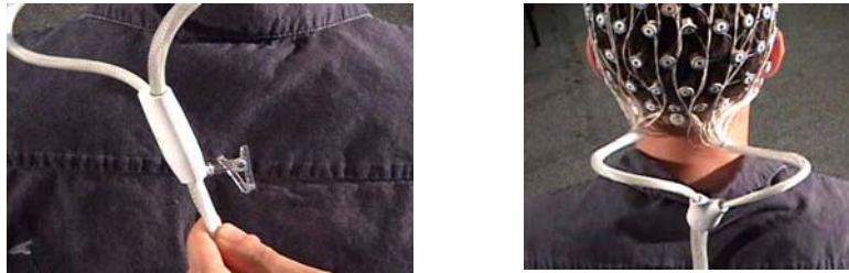
Figure 6-21. Secure the Y clip to the collar
