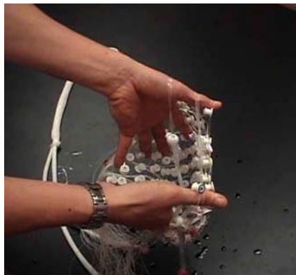
Figure 6-9. Stretch the perimeter band with thumbs and little fingers
