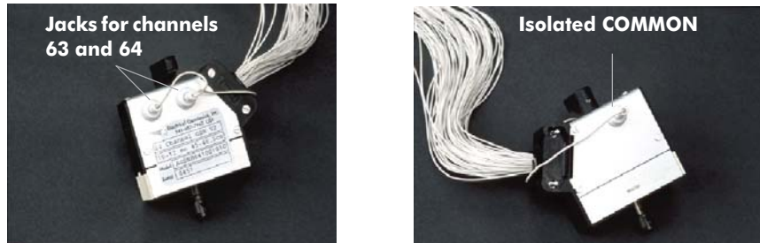
Figure 3-9. Infant Net special Hypertronics connector, with outrider jacks strapped to isolated common
