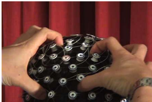
Figure 6-15. Adjust Net position by grabbing large sections and shifting them uniformly
