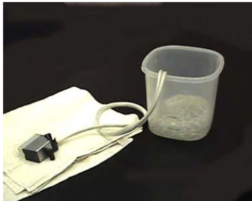
Figure 6-5. Placing the sensor end of the Net in the electrolyte bucket
