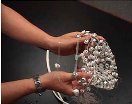
Figure 6-8. Place thumbs under the Net's perimeter band
