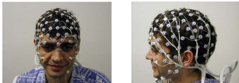
Figure 2-1. 128-channel HCGSN, front (left) and side (right) views
