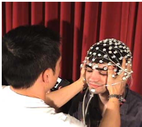
Figure 6-11. Check position of Net before disengaging your hands
