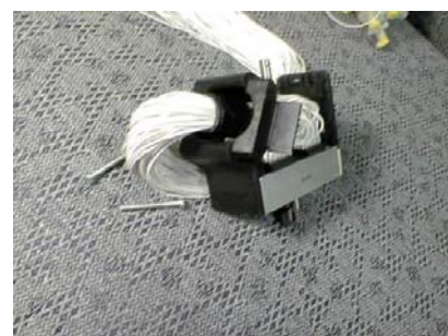
Figure 9-5. Remove the screws and slide the clamp out
