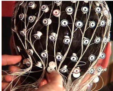
Figure 6-13. Upturn tilted sensors; check the back of the head
