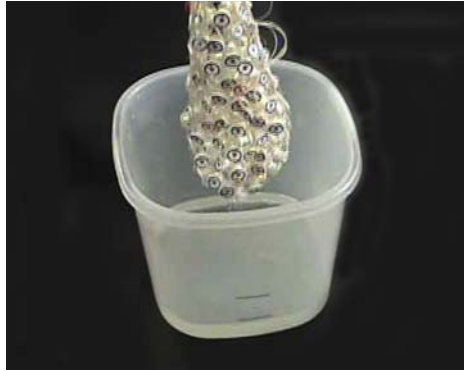
Figure 6-6. Lifting the Net out of the electrolyte bucket
