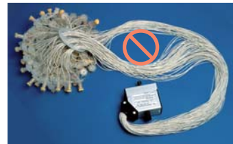
Figure 3-11. Avoid passing connector or sensor end of GSN 200 through lead bundle
