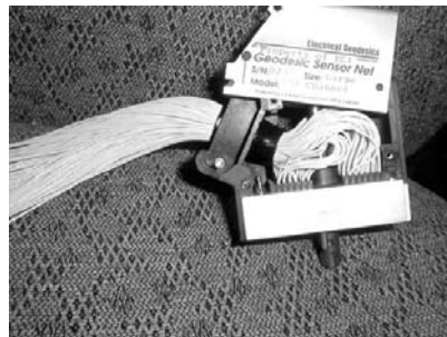
Figure 9-14. Replace the hood without crimping the wires
