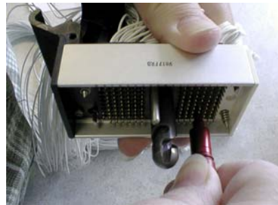
Figure 9-10. Push the tool until the contact pin slides out
