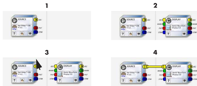
Figure 3-24. Cabling two devices together
